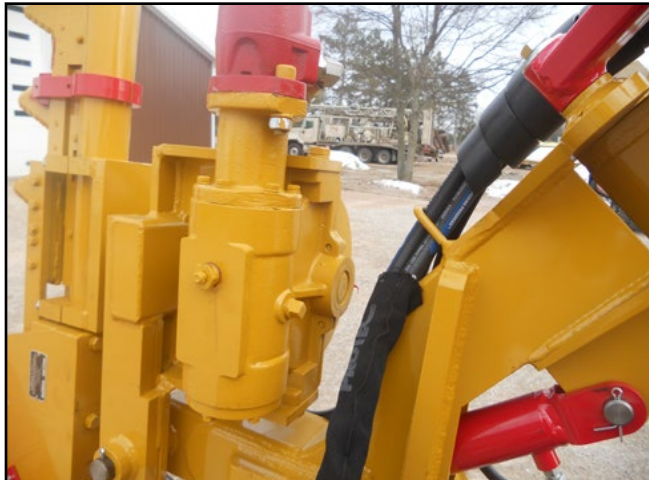
FIG 17 E Check pump drive gearbox gear-lube daily and change every 400 hours.
