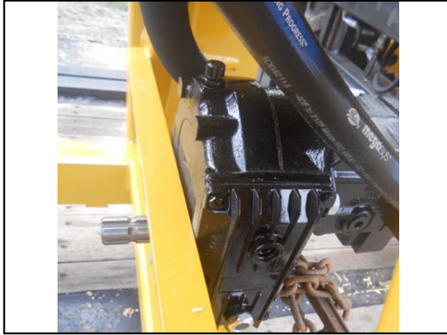
FIG 17 D Check rotate gearbox oil level every 200 hours, change every 400 hours of operation. Use 10W-90 Gear Lube
