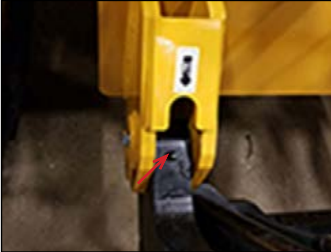
Mast grease point. There are 2.
