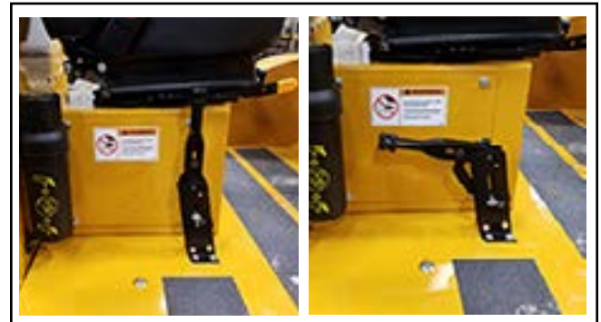
Engaged FIG. 23 Disengaged
