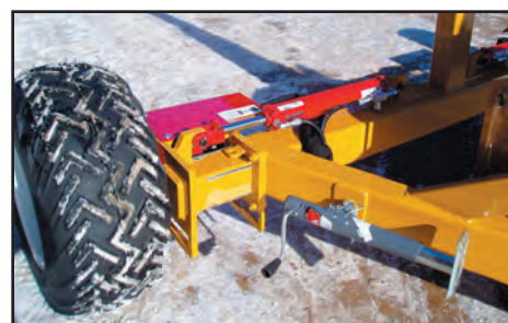
Optional hydraulic sliding axle for 25' lift.
